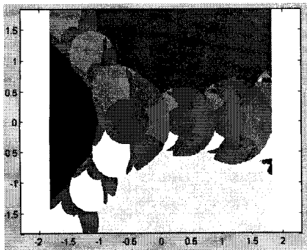
This image shades each point in the plane according to which roots it goes to on iteration of the self-consistent roots method.
